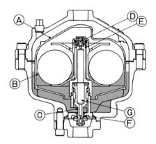
When the condensate level in the trap body rises to a certain point, the floats (B) rise. This, together with the help of the coil spring (E), lifts the float holder, causing the pilot valve (D) to open.
