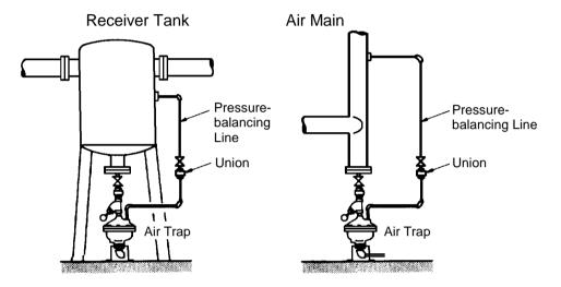
Note: Be sure to connect the pressure-balancing line to an area with the same pressure or to an air section downstream of the flow medium.
